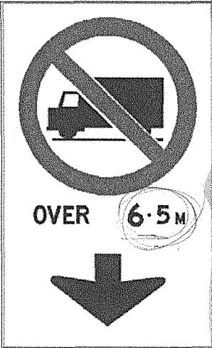
LANE USE RESTRICTION Sign (Length-based, Overhead) RB-40 90X150CM ENGINEER GRADE (ADDED-NEW)
